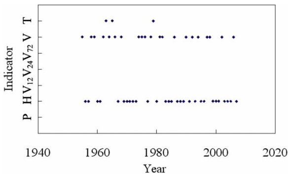
Figure 6 | The indicator corresponding to the maximum contribution rate in the same flood process. P: peak flood discharge; H: peak level; V12: the maximum 12-h volume; V24: the maximum 24-h volume; V72: the maximum 72-h volume; V: the total flood volume; T: flood duration.
